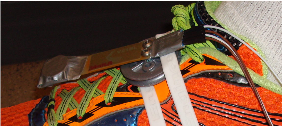
Figure 6.4: Foot mounted piezoelectric testing setup
