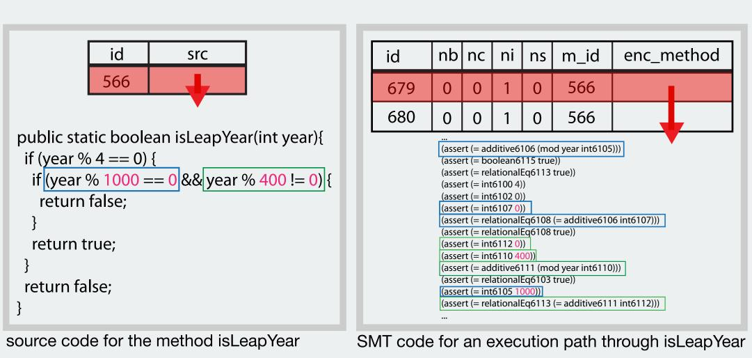
The method 'isLeapYear' has two execution paths, stored as separate database entries. Each path is encoded in SMT as a set of first order logic expressions. After binding the IOPair to the encoded path, **Z3** can determine if the path will satisfy the IOPair specification.
