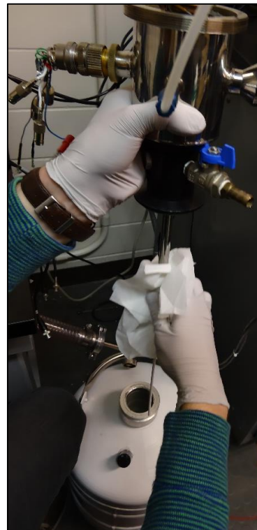
Figure 16: Wiping the condensation from the tube before reinserting it.
