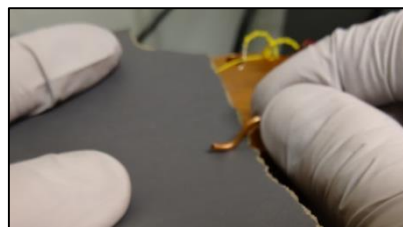
Figure 4: Sanding the underside of the clamp
