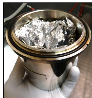
Figure 2: Aluminized mylar packed into the top cover of the vacuum chamber, leaving enough space for the shroud
