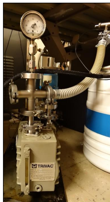
Figure 12: The vacuum pump. Ensure that the oil levels (visible on the bottom left) is within the recommended limits.
