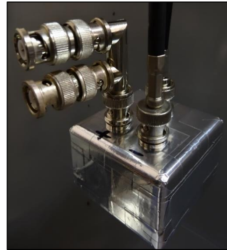
Figure 10: The shielded junction box with the connectors and adapters
