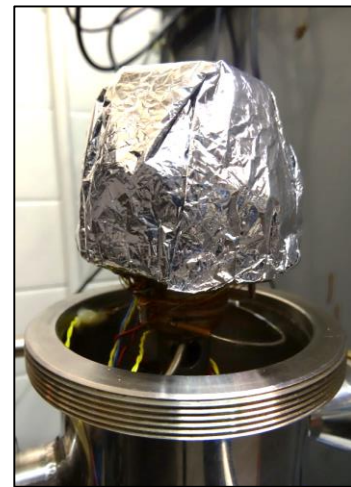
Figure 7: The shroud on the cryostat
