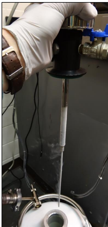
Figure 15: Extracting the tube from the flask. The tube is still dangerously cold.
