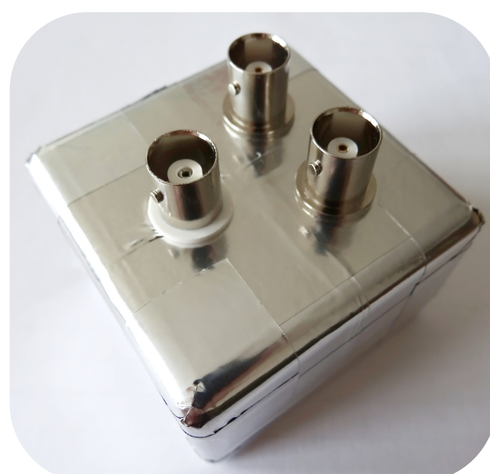
A custom-built low-noise junction box for the picoammeter and the voltage source
