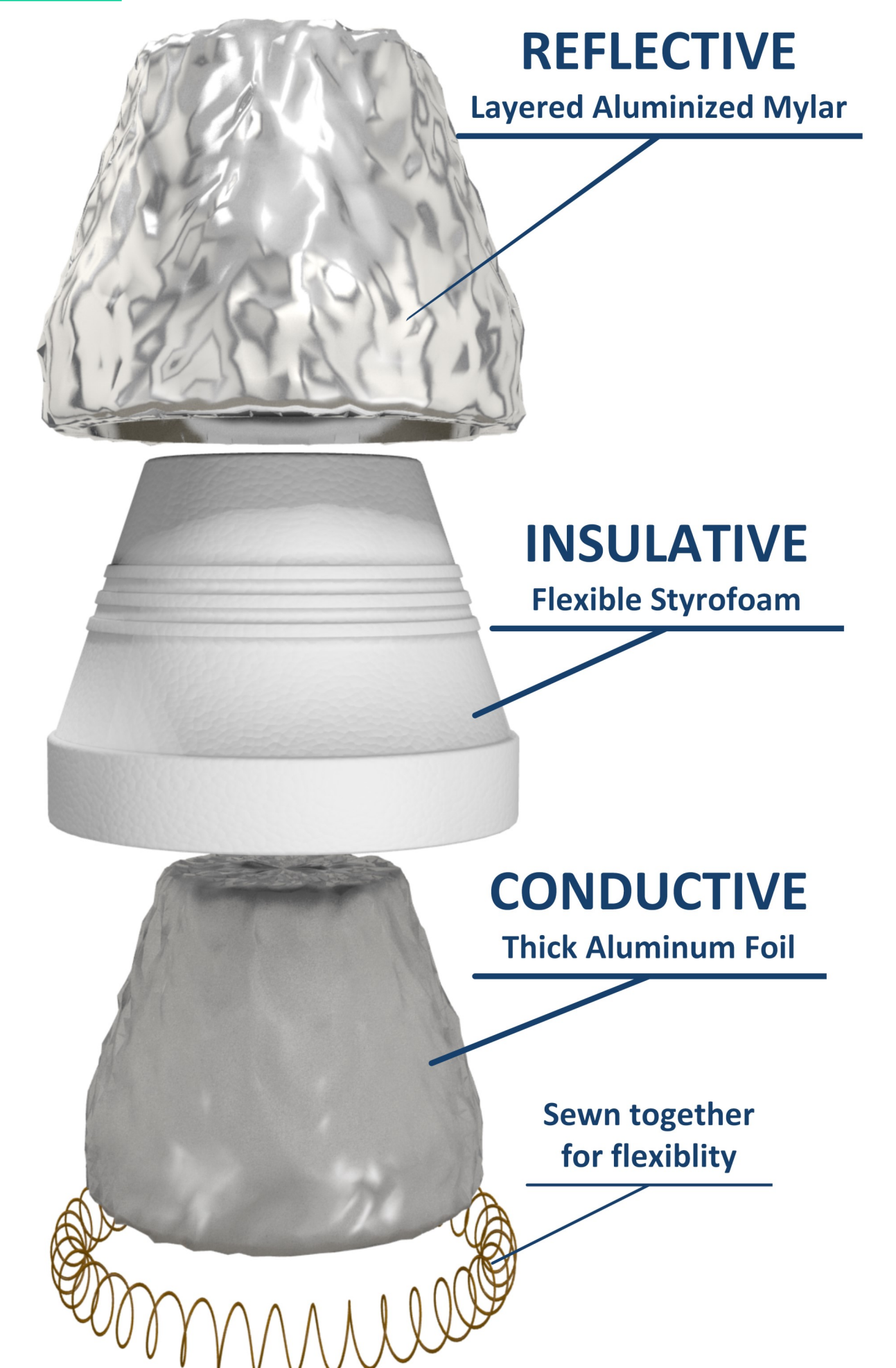
The layered shroud prevents all kinds of thermal loss
