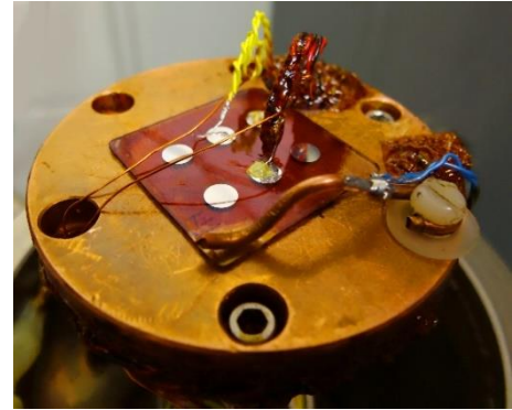
Figure 4: Photograph of the cryostat, with a sample loaded and ready to be tested
