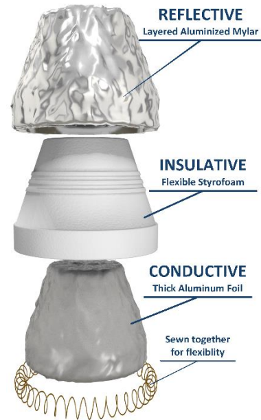
Figure 7: Exploded view of the layers involved in the shroud
