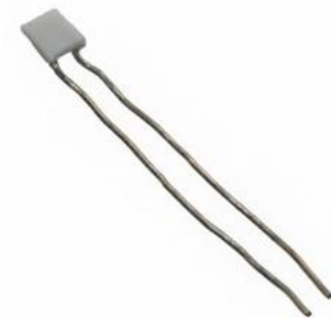
Figure 5: Magnified image of the RTD sensor. The white rectangle is roughly 1 mm on a side.
