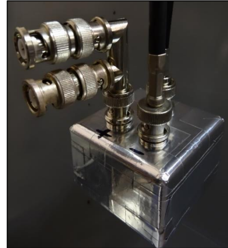
Figure 28: The shielded junction box with the connectors and adapters
