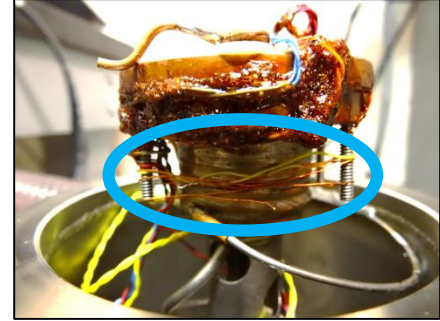
Figure 24: Stabilizing the tie-down wires by wrapping them around the screws on the
