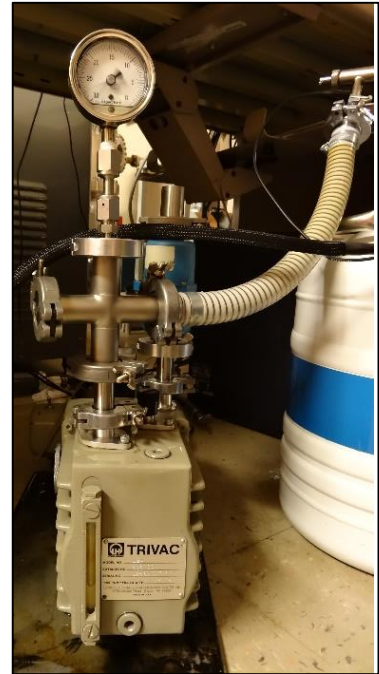
Figure 30: The vacuum pump. Ensure that the oil levels (visible on the bottom left) is within the recommended limits.
