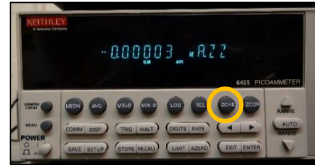
Figure 27: The 6485 Picoammeter front panel, with the position of the ZCHK button marked.
