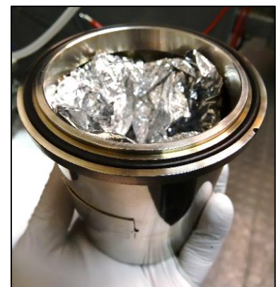
Figure 20: Aluminized mylar packed into the top cover of the vacuum chamber, leaving enough space for the
