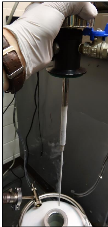
Figure 33: Extracting the tube from the flask. The tube is still dangerously cold.
