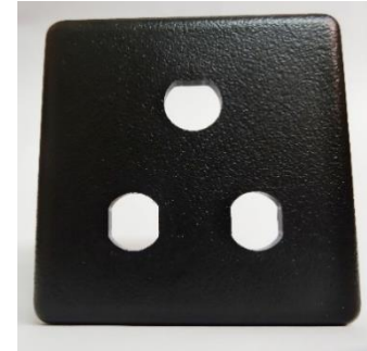
Figure 11: The ABS plastic box after being machined
