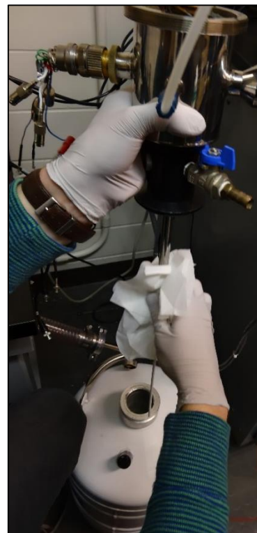
Figure 34: Wiping the condensation from the tube before reinserting it.
