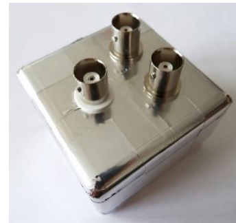
Figure 12: The completed shielded junction box
