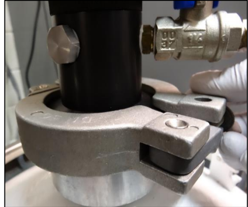
Figure 32: Opening the collar to remove the flask
