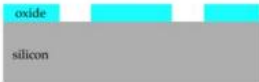
Photoresist is washed away using acetone
