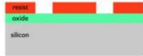
Removal of exposed photoresist by developer
