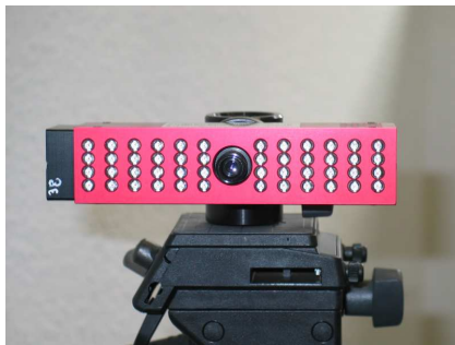
Figure 1. Swissranger SR2 and its technical specification (taken from [12])
