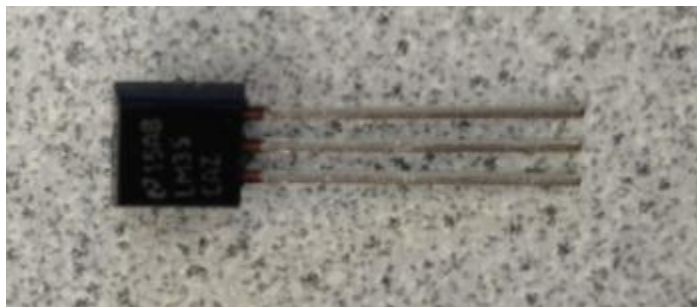
Figure 5: TI LM35 Temperature Sensor
