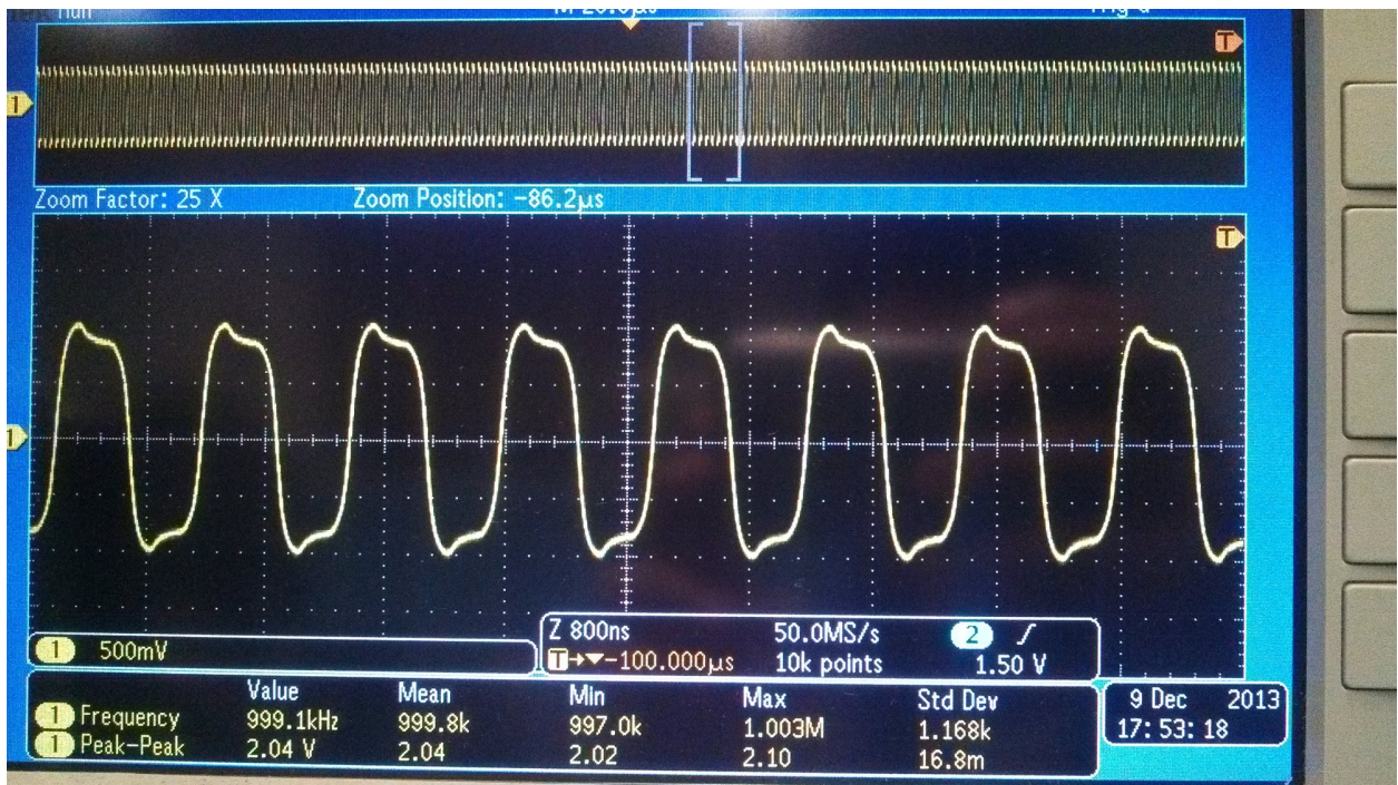
Figure 19: Output waveform of 5v input
