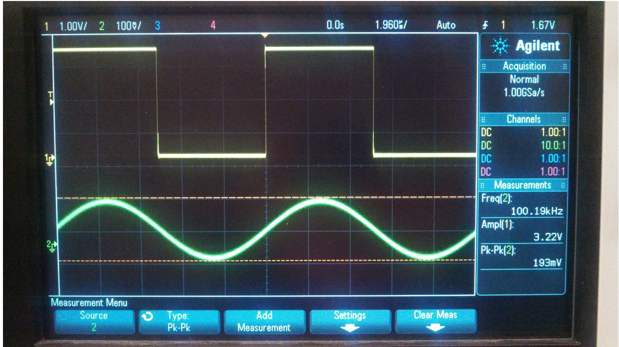
Figure 18: Output waveform of 200mv input sine wave along with trigger signal
