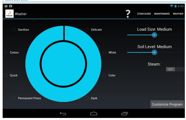
The Washing Machine Application opens with the wash program settings screen. On the left, is a dial controlled by finger movement in the outer ring, which is used to select the wash program. Selecting the center of the dial starts the currently selected wash program. On the right, are slider selectors used to select load Size and Soil Level as well as a switch to turn steam on and off. In the lower right, is a navigation option to move to the customization screen.
