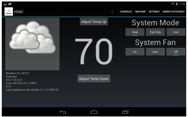
This is the main screen for the HVAC system. It is the screen that initially appears to the user and is the base for many basic functions. The home screen allows the user to view the current temperature, adjust the temperature up or down, check the current weather, set the HVAC system settings to Heat, Fan, or Cool and On, Auto, or Off.
