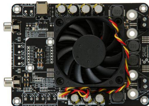
2x50 Watt Stereo Class-D TDA7492 Amplifier Board
